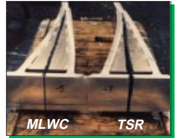
Reduced Weld Distortion 70%. Grumman Aerospace.
