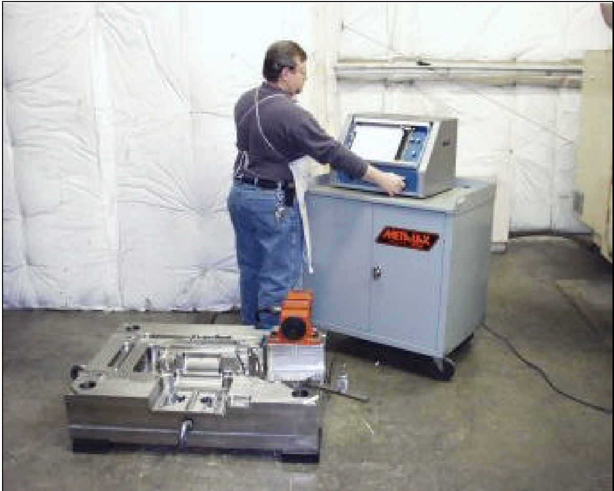
Figure 1. Minco Tool and Mold, Dayton, OH, has an ‘on time every time’ delivery policy. Sub-harmonic stress relieving plays an important part of this commitment in limiting stress relief to two hours. In doing so, they also realized elimination of most costs associated with heat treat stress relief and yet they maintain their high standard of quality.
