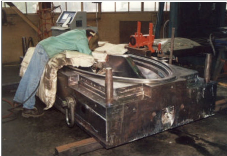
Figure 9. Modern Tooling Systems, Toledo, OH, impressed their customer when they put over 80 hours of welding on this 25,000 lb. P20 jet ski mold without cracking. The key was sub-harmonic stress relief during welding. Without sub-harmonic energy they had cracking within 15 seconds. The extensive engineering change turned out to be no big deal.
