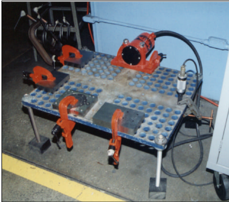
Figure 6. Hydro-Cam and Engineering, Troy, MI, eliminated a 56% scrap rate on a unique design for carbide preform dies. Applying the sub-harmonic vibration treatment immediately before wire EDM was the key. It's the law now. Sub-harmonic processing saves their customers a substantial amount of money.
