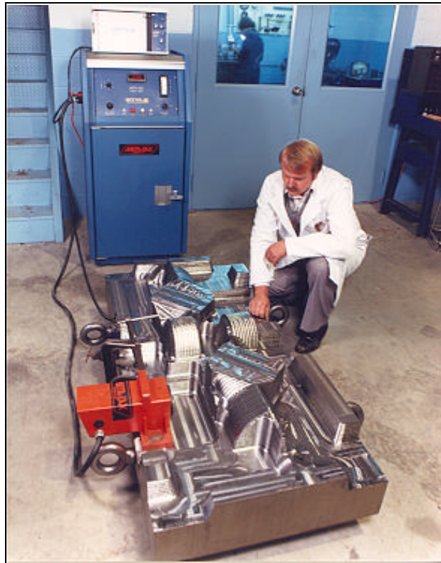
Figure 2. Build-A-Mold, Ontario, Canada, has used sub-harmonic vibrations for stress relief since 1986. They have noticed that their production is smoother and their customers have noticed the service life of their molds have improved, sometimes up to double.
