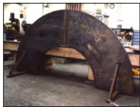
10 foot diameter disk after welding.
